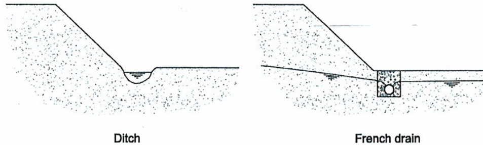
Figure 3.5 Ditch and French Drain
